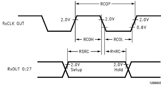
FIGURE 8. DS90CF364 (Receiver) Setup/Hold and High/Low Times
