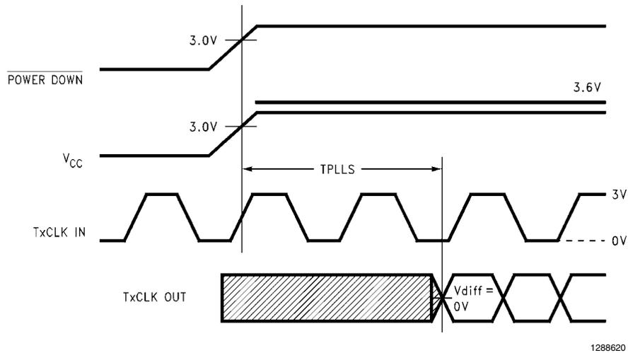
FIGURE 11. DS90C363 (Transmitter) Phase Lock Loop Set Time
