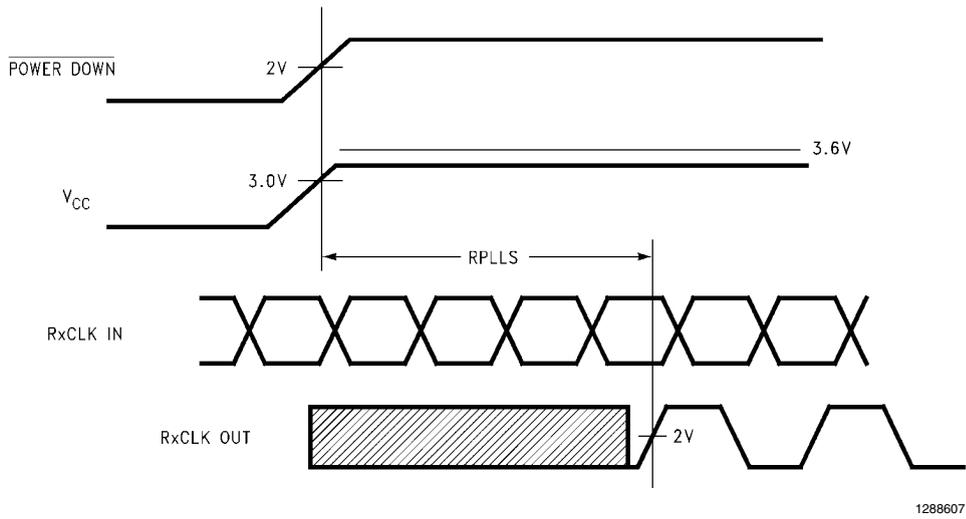
FIGURE 12. DS90CF364 (Receiver) Phase Lock Loop Set Time
