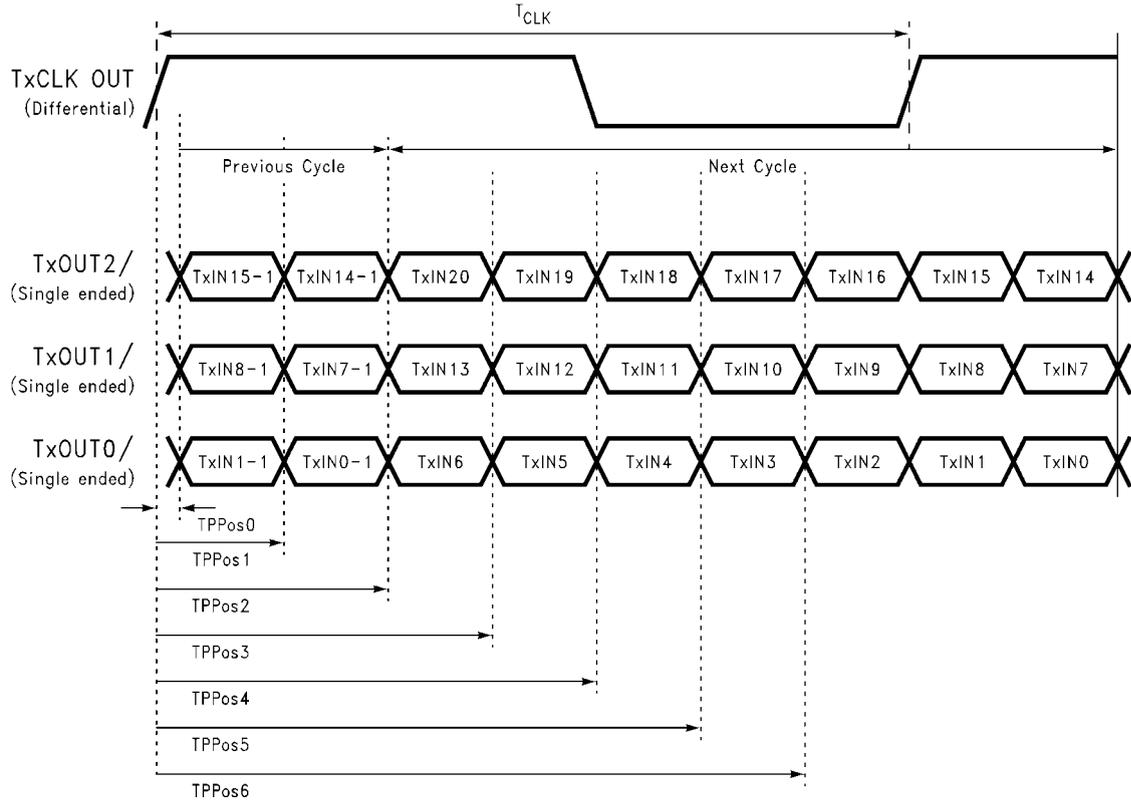
FIGURE 17. Transmitter LVDS Output Pulse Position Measurement
