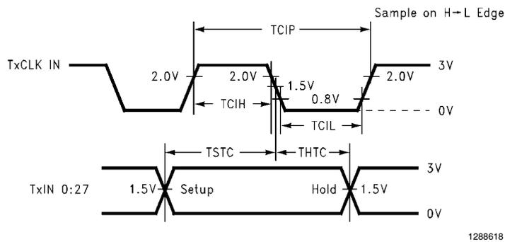
FIGURE 7. DS90C363 (Transmitter) Setup/Hold and High/Low Times
