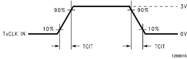
FIGURE 5. DS90C363 (Transmitter) Input Clock Transition Time
